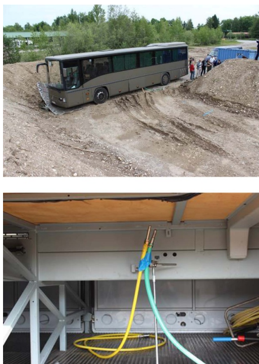
Figure 1. Setup of the field experiment: The Ir-192 source is placed in the baggage compartment of the bus, similar as it was the case during the Cochabamba incident (top). Location of the sources inside the baggage compartment of the bus. The end tips of the guidance tubes of both Ir-192 sources (0.65 and 1.5 TBq) were simultaneously fixed on a tripod to ensure similar exposure conditions, regardless of which source was currently being used during the experiment (bottom). The end tips were closer to the seating floor than in the IAEA reconstruction of the Cochabamba incident, in order to maximise the dose to the fortuitous dosimeters.
